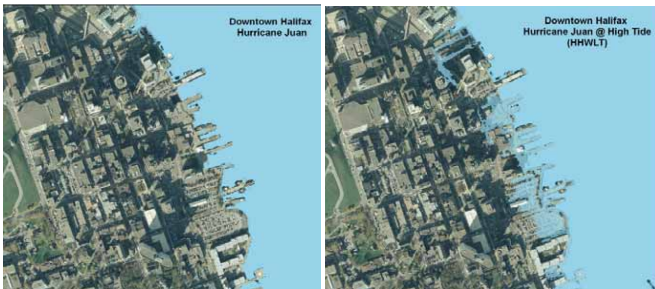
Figure 7.7: Flooding scenarios for downtown Halifax. The peak water level during Hurricane Juan was 2.9 m chart datum (left panel). It could have been 3.4 m had the surge coincided with the high tide 2 hours earlier, or it could have been 3.6 m (right panel) had it coincided with the 'higher high water large tide' (the average of the 19 annual predicted highest high waters) (Source: Manson et al. , 2008).
